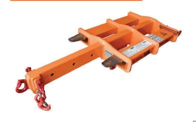
Multi-position forklift that can be removed and takes up little space. In the lower part of the equipment there is a multi-hole band for the assembly of a special shackle with a swivel hook. Each hole has an overall capacity equal to the maximum allowed and more holes can be used, dividing the load. The forklift is equipped with a removable arm, adjustable in different positions by inserting a pin in the appropriate seats.
