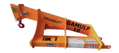
the forklift attachment consists of a fixed structure with a removable arm, which can have one or more adjustment positions. The extension can be adjusted by inserting a pin in the appropriate seats. At the end of the arm there is a swivel hook fixed by a pin.
